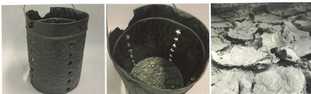
Above, figure 4: Inside and outside view of the 30-litre drum after pyrohydrolysis test as well as dust remains in the drip tray
